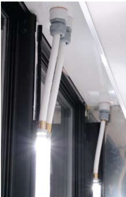
The side emitting rods shown mounted inside a cabinet
